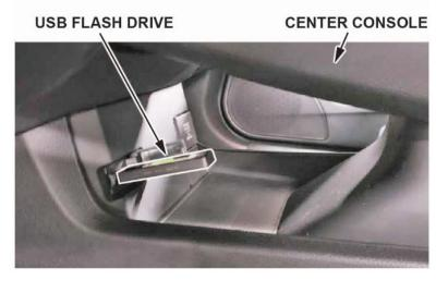
The audio unit will automatically detect the USB flash drive and start the update process.
