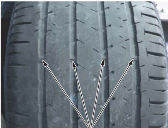
EXCESSIVE EVEN WEAR
