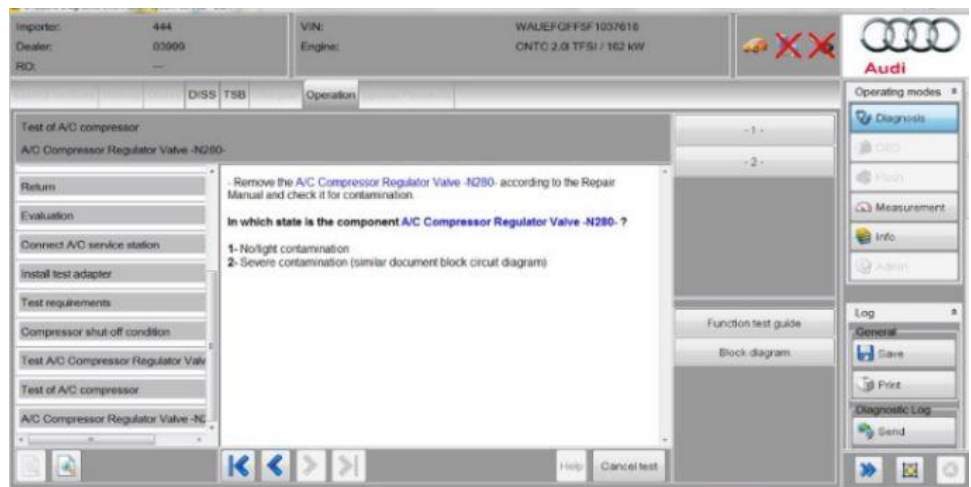
Figure 9. Checking for N280 valve contamination.
