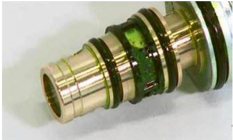
Figure 11. Severe contamination at the N280 valve filter screen.
