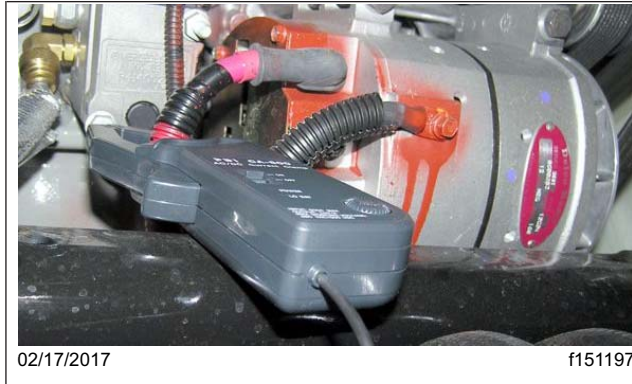
Fig. 13, Use an amp clamp around the positive alternator cable to measure the draw of the carbon pile.
