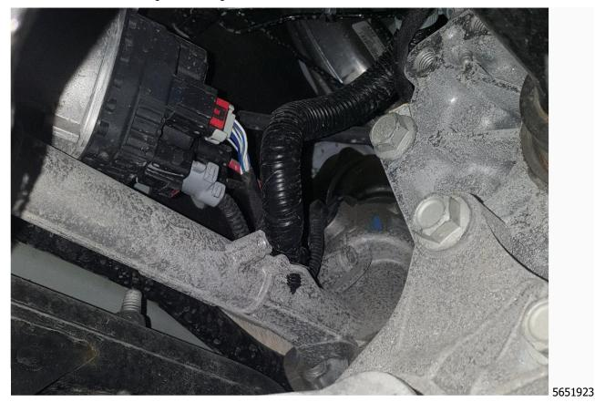
2. Inspect the engine harness branch where it clips into the Power Steering rack as shown.
