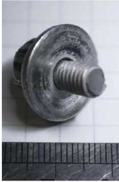
Fig. 4 Broken AMP Bolt Remnants
