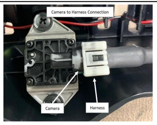
**Repair**: Fully disengage and reengage the connector to confirm it is fully seated.
