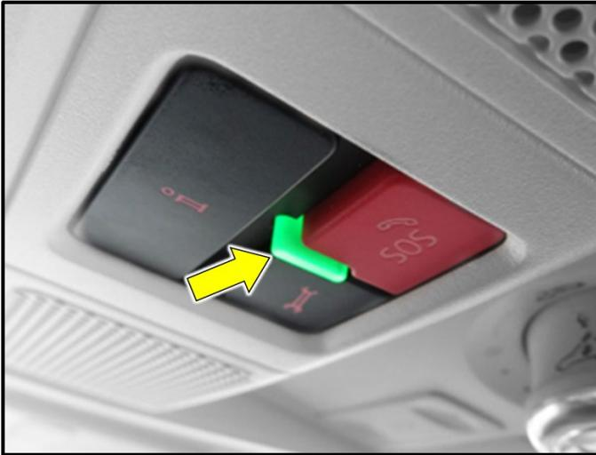
Check the status of the status light <arrow> in the Car-Net button array:
