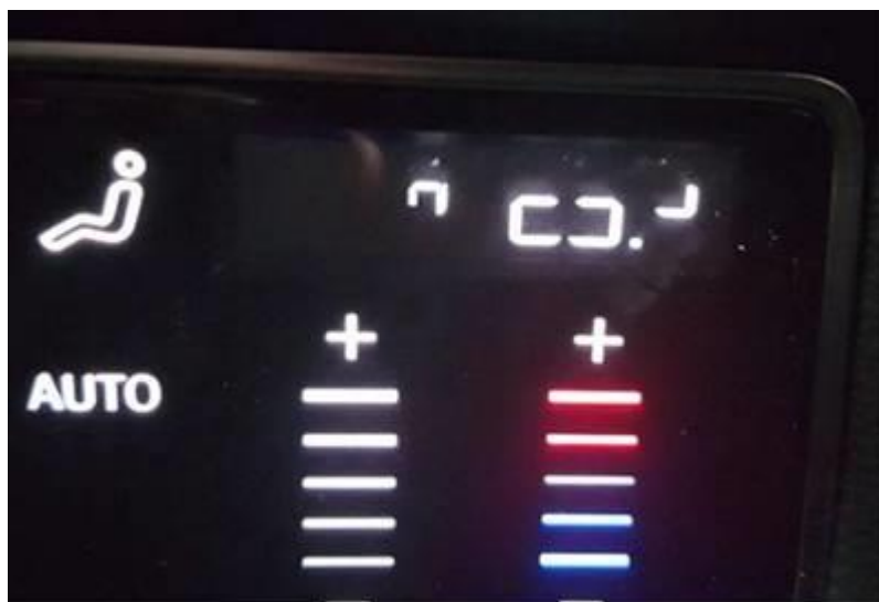
Figure 1. Rear A/C control display E265 with missing readout segments.
