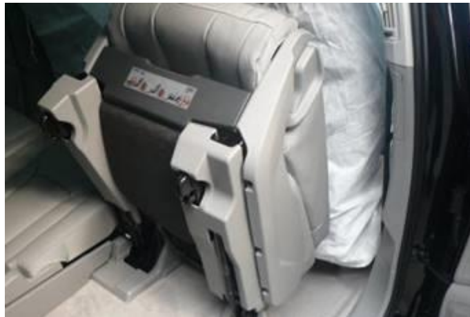
Figure 2. Affected seat unlatched and tilted forward.
