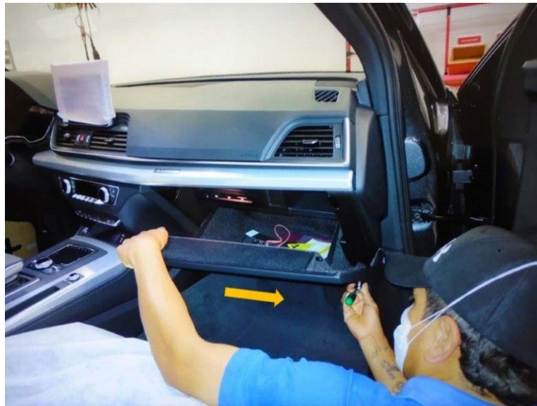
Figure 2. Adjusting the glove box to increase clearances.
