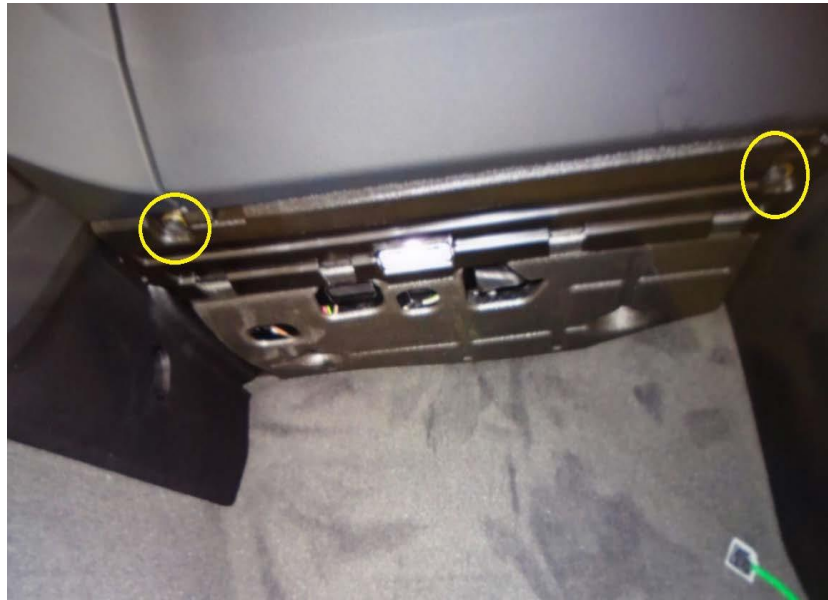
Figure 1. Both lower glove box bolts.
