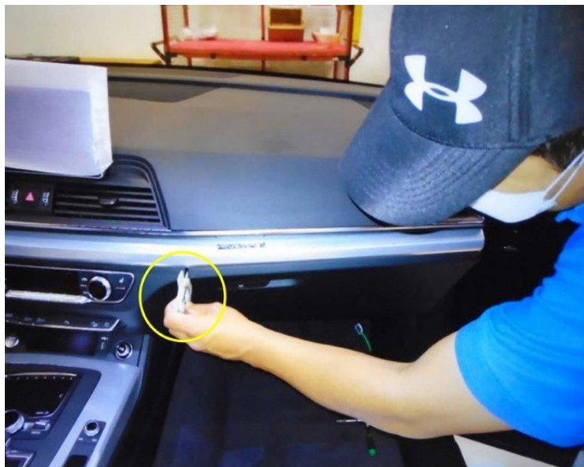
Figure 3. Checking the gap between the glove box door and the center console.
