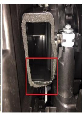
Not OK: Blower Assembly foam insulation found rolled, not positioned in correct, location allowing air to leak.
