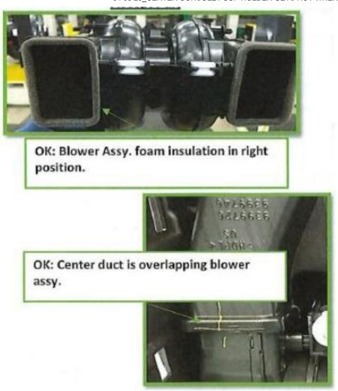
2. Check if the foam material to the next connecting piece is correctly installed. If damaged install a locally sourced, one side self-adhesive
