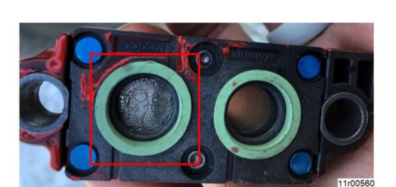
Figure 1, Condensation on the EGR Differential Pressure Sensor.
