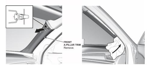
15. Remove the driver's and passenger's upper trim, then remove the upper dashboard trim.
