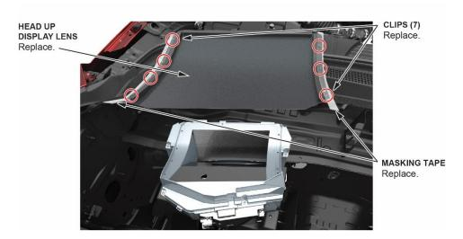
19. Make sure the lens is set onto the locator pins. Push the seven clips in by hand or by using an angled needle-nose plier to set them in place, then remove the masking tape.
