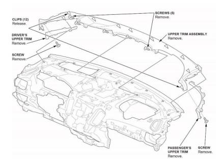
16. Apply masking tape on the back of each clip to hold them in place during removal.
