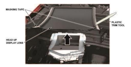
18. Install the new clips with new masking tape holding them in place while installing the new HUD Lens.
