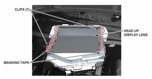
17. Remove the lens by pulling up on the edge using a plastic trim tool.
