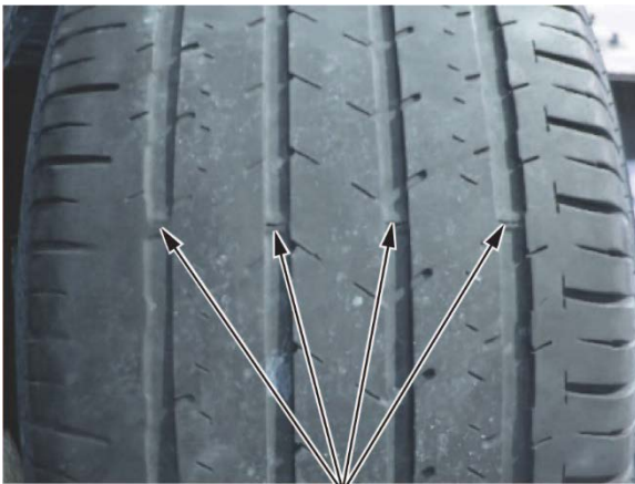
EXCESSIVE EVEN WEAR
