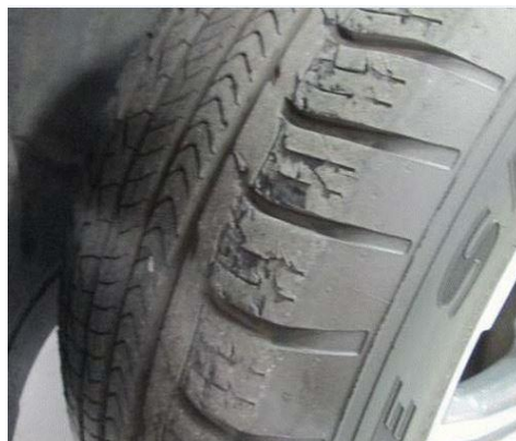
Figure 1. Irregularity on the outer side and on the inner side of the tire.
