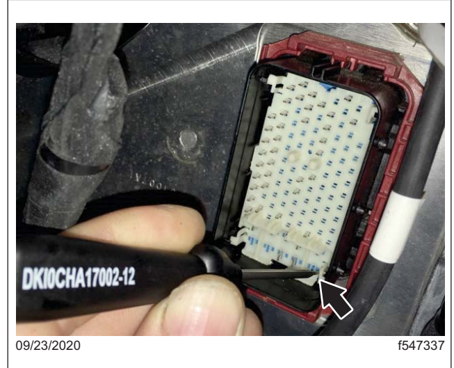
Fig. 8, Using the Hook to Lift the Stabilizer Plate into Pre-Stage Position
