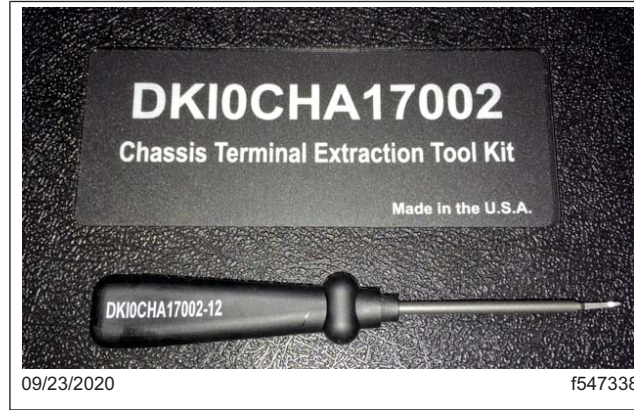
Fig. 3, Tool for Resetting the Terminal Stabilizer Plate Locks
