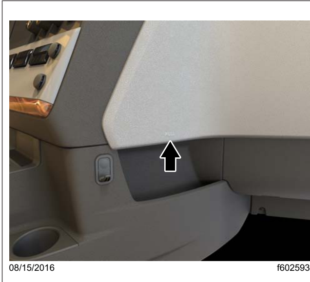
Fig. 1, Electrical Bay Cover Handhold
