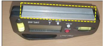
To initialize angle measurements, set the protractor against a reference surface. When the reference position is set, press the **All Zero** button to set to zero (0).
