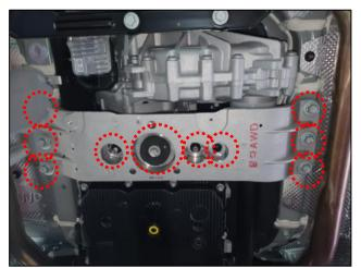
7c. Install the washers above the T/M mounting bracket and the insulator.
