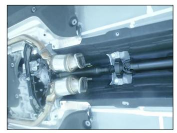
2. Place and hold the protractor to the transmission LH flange face to set the transmission reference angle to zero (0.0).
