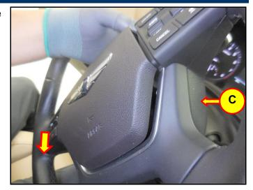
8. Turn the steering wheel to return it to upside position. Slightly lift the DAB outward (D).
