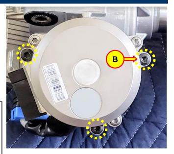
6. Remove the motor assembly (C).
