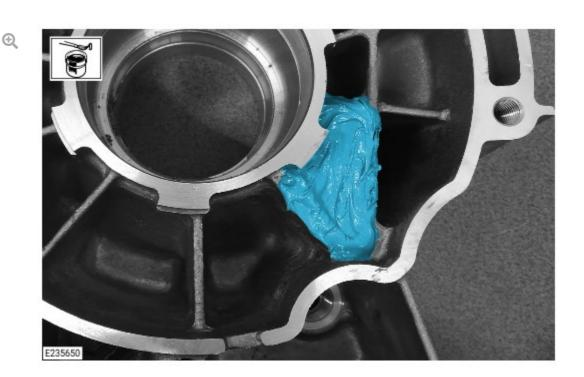
Apply an even layer of Devcon putty to the transmission insert until it is completely filled and covered.
