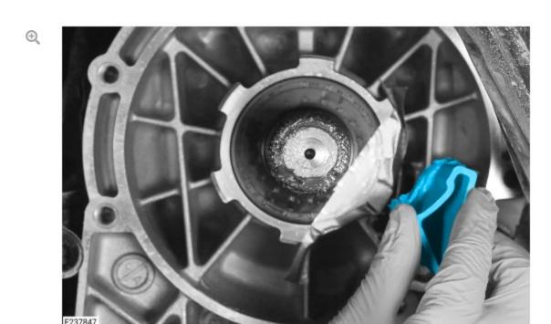
Use a suitable tool to push the transmission insert into the area shown.
