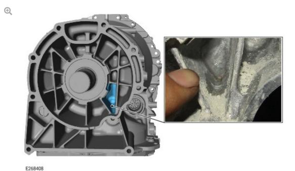
This technical bulletin only applies to vehicles installed with the 8HP45 8-speed All Wheel Drive (AWD) automatic transmission, with oil diagnosed to be leaking from the cavity highlighted in the illustration.
