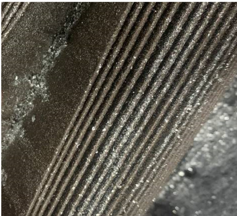
Figure 4 Example of a filter with a separated seam
