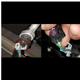
Example of a Connector with Damage Terminals Backed Out and the Location of the Connector
