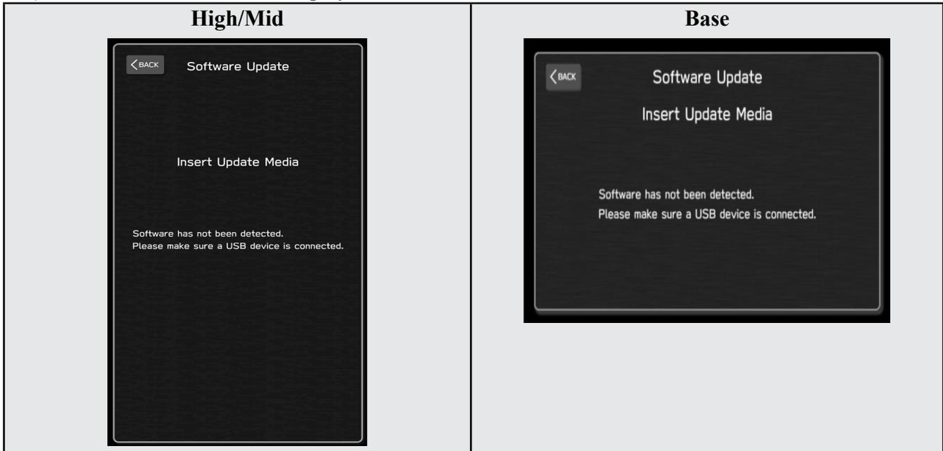
4e) Insert the H/U reprogramming USB into the USB port and press **OK**.
