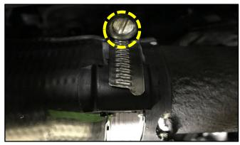
2a. Confirm that the hose clamp (A) break away nut head (B) is not present. If so, this action is complete.
