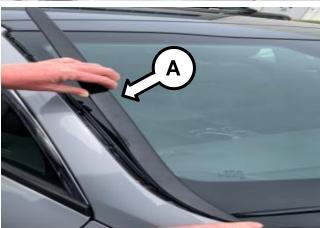
3. After the top is fully seated work your way down the trim piece seating it fully until you reach the bottom.
