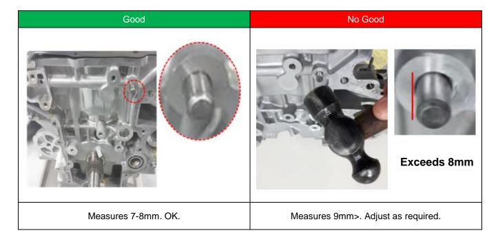
Note: <u>If the dowel pin measures less than 6mm</u>, replace the engine block due to incorrect drilling depth. <u>Confirm proper authorizations prior to block replacement</u>.
