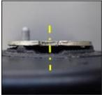
When looking at the mounting rubber off the vehicle, the metal bracket recesses should be aligned to the corresponding indicators on the rubber part.
