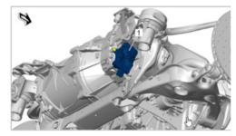
Figure 1 - ETSM (1) Location on Transmission
