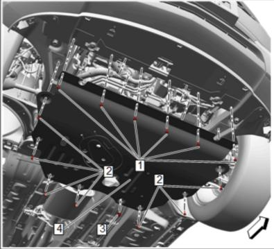
1. Remove the front compartment insulator (Base). Refer to Front Compartment Insulator Replacement (Base) in SI.
