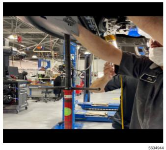
3. Push up on the CRFM slightly so you can move the bushing holder forward within the vehicle, then out the bottom.
