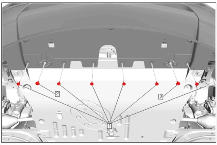
5. Reinstall the six front bumper fascia extension bolts (1) and the two front bumper fascia extension retainers (2).
