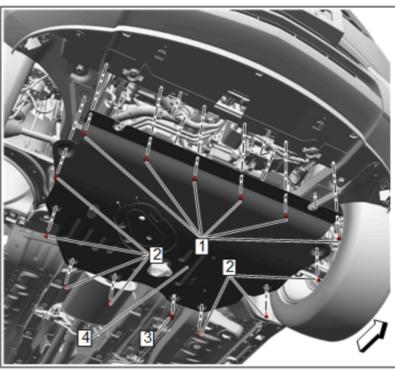
6. Reinstall the front compartment insulator (Base). Refer to *Front Compartment Insulator Replacement (Base)* in SI.
