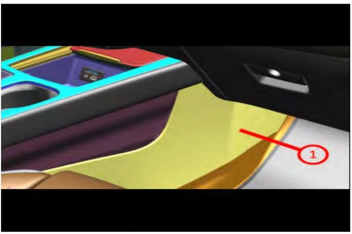
3. The front floor console extension panel (1) needs to be removed to gain access to the running wire. Refer to Front Floor Console Extension Panel Replacement - Right Side in SI.
