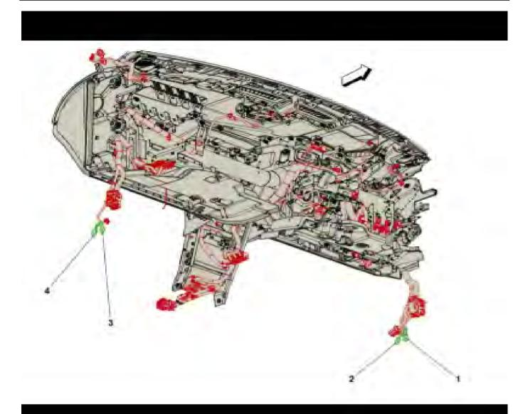
2. Cut the terminal 3 black ground wire from the USB HUB and butt connect to the USB HUB a new 0.75 mm jumper wire about 2600 mm (8.5 feet) in length. Run the wire behind the instrument panel and carpet to Ground 202 (3), located on the passenger side of the vehicle. Cut back and tape off the original ground wire with electrical tape.
