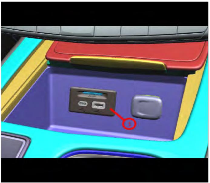
1. Partially remove the USB HUB (1). Follow the Multimedia Receptacle Replacement in SI to get to the back and locate the USB HUB ground wire. 5537651
