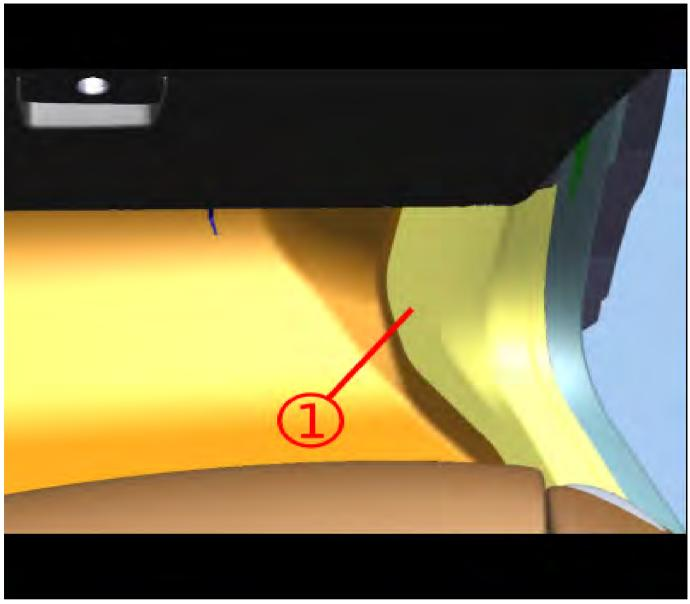
4. The front passenger-side door sill panel (1) needs to be removed to gain access to the running wire. Refer to Front Side Door Sill Garnish Molding Replacement in SI.
