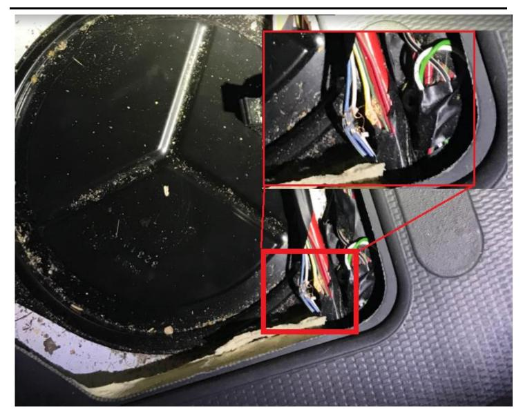
**Repair**: Repair the wiring as necessary using standard procedures. Reroute the harness away from the access panel lock tab. Be sure it is routed in a way that the circuits can no longer be damaged.
