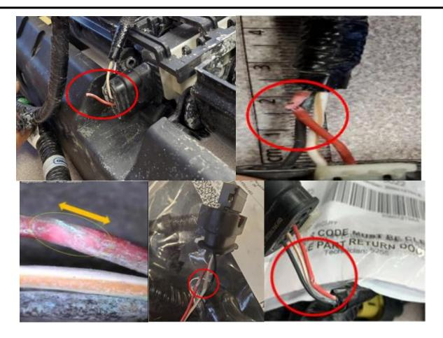
**Repair**: Use wiring kit 68396618AB to repair the fascia wiring harness or replace the harness as necessary. If corrosion is present in the AGS connector, replace the AGS and AGS Connector
