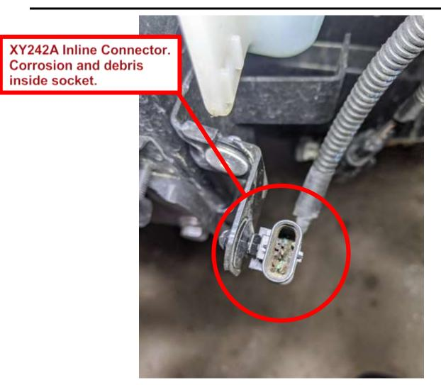
**Repair**: Cut and discard the connector. Cut back the wiring harness until there is no longer corrosion found. Using heat shrink, individually isolate and terminate each of the three circuits. The three circuits cannot be allowed to touch each other or chassis ground. Using zip ties or similar, tie back the harness so it does not create any issues in the future.
