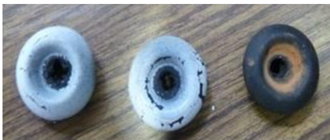
Figure 3. Modified sill plugs with 6mm hole drilled.
