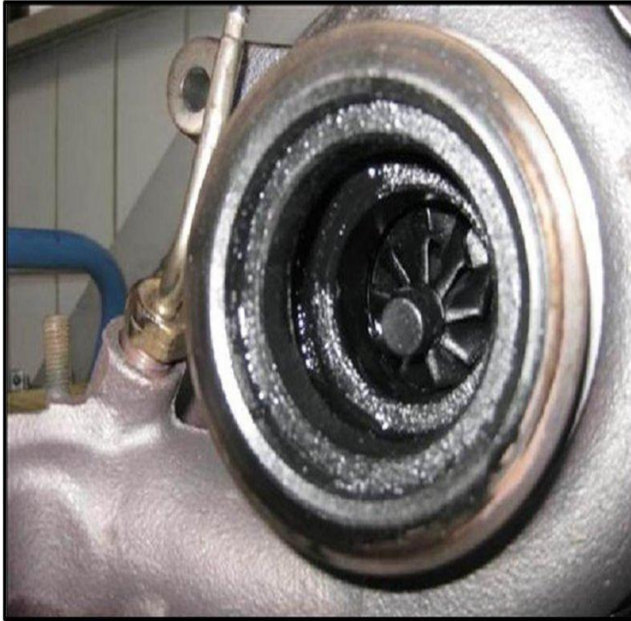
Figure 1 (broken turbocharger shaft, engine oil ingress on exhaust side).
