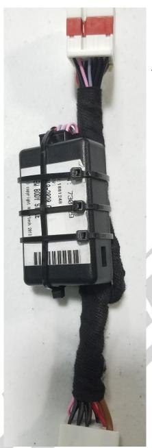
The final cable tie installation should result in a harness/module package as shown here which is ready for installation. This ensures a tight and permanent connection which is resistant to vibration.
