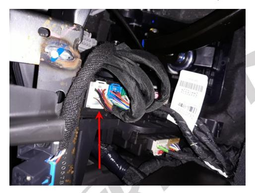
2. Plug the male end of the Inline Speedometer Module Harness into the female end of the OE Harness.
