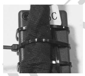
The fourth cable tie should be routed around the module to secure it firmly to the harness.
