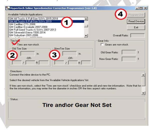
2. For accurate readings, measure the stock and new tire height from the ground to the top of the tire. Enter these measurements (in inches) into the configuration software, and click program to commit these settings. Once configuration is complete, take the Speedometer Calibrator module and harness to the vehicle.
