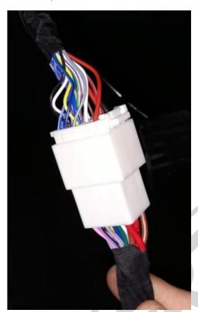
Fully connect the Speedometer Calibrator harness's male connector to the factory harness which was unplugged from the BCM. Ensure the connector is fully seated and locked into place.
