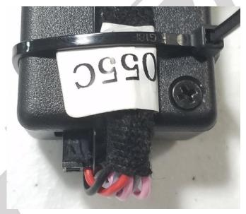
The second cable tie should be routed near the connector to eliminate harness movement near the connector without blocking access to the USB connector on the side.
