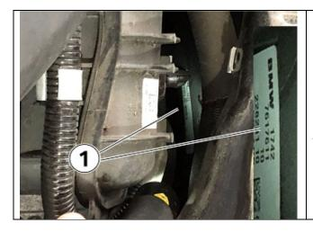
**Important**: In conjunction with replacing the radiator as outlined in Situation A, check the part number of the fan shroud (1).
