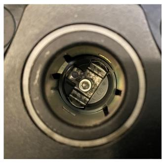
4. Insert the replacement bolt and hand tighten (McMASTER-CARR, item number 91292A112).
