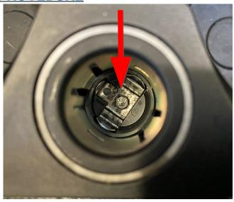
1. Remove the fuse that powers the front 12 V power socket. Fuse number and location can be found in ISTA or AIR.
