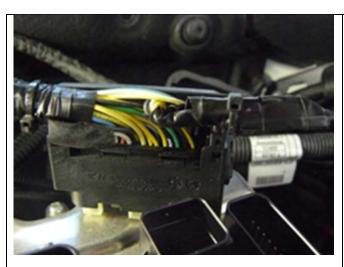
Splice the new harness to the existing wiring in connector A46\*2B, using the supplied splice crimp connectors and heat-shrink tubing.
