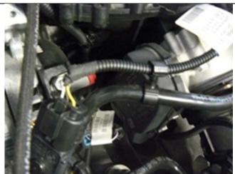
The replacement harness is then secured to the plastic ventilation pipe with the clip.
