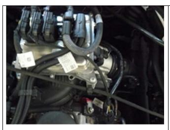
Remove the engine acoustic cover to access the DME harness connectors.
