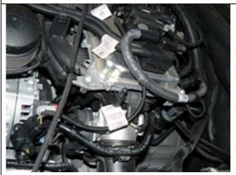
Reconnect the DME harnesses and reinstall the engine acoustic cover.
