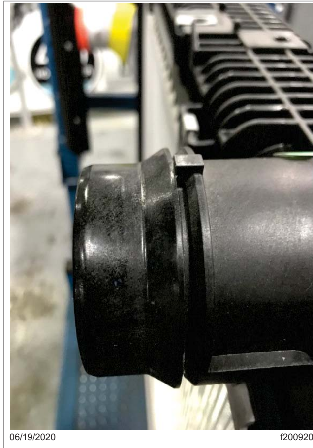
Fig. 5, Upper Radiator Hose Removed
