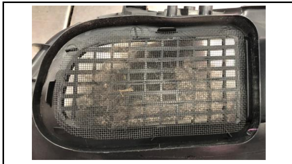
Figure 5. Example of a Dirty RAV4 HV Battery Cooling Intake Filter
