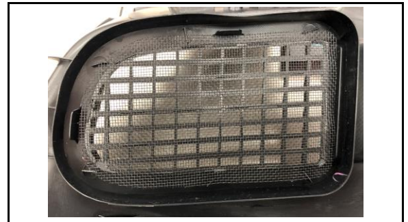
Figure 6. Example of a Clean RAV4 HV Battery Cooling Intake Filter
