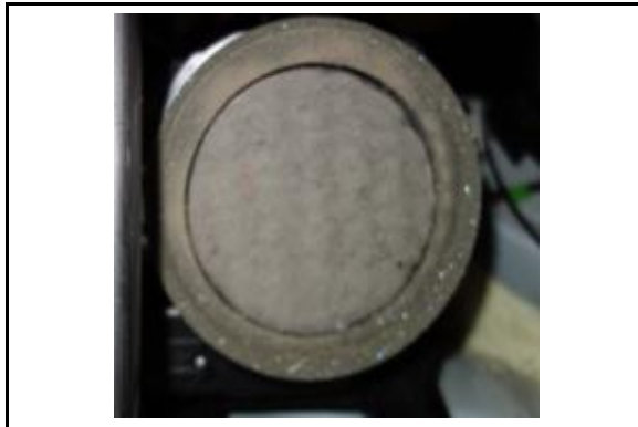
Figure 3. Example of a Dirty Prius C HV Battery Cooling Intake Filter
