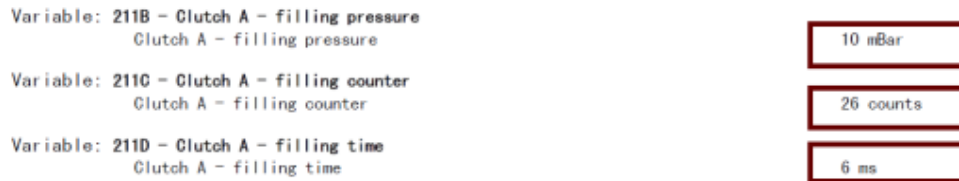
Figure 6: Clutch Filling Counters in the ENGINEERING PARAMETERS in the TCM module.
