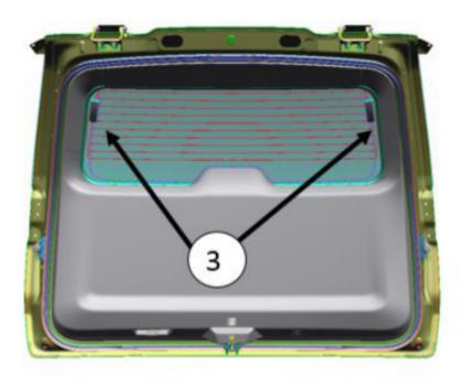
3. With the liftglass open, inspect to ensure that all fasteners that attach the spoiler to the liftglass are torqued properly. See doc ID 5601125 for all the spoiler's fastener torque specs.
