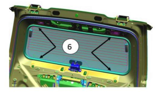
6. With the liftgate closed, push on the liftgate near the bottom as shown (7) to see if it feels soft/loose. If the liftgate has for/aft movement then adjust the liftgate striker forward 1.0mm using the steps below:
