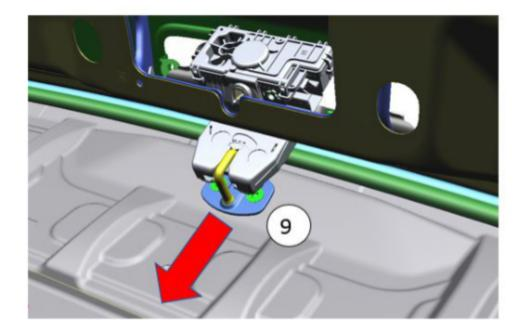
7. Inspect the liftgate strike to make sure it is centered in the liftgate latch opening (10). Observe the liftgate striker for wear on one side of the striker. In most cases, wear marks will be seen on the driver's side of the striker. If this is the case, loosen and adjust the striker to the passenger side 2 mm and tighten fastener to 22 Nm (16 lb ft). Adjust as necessary.
