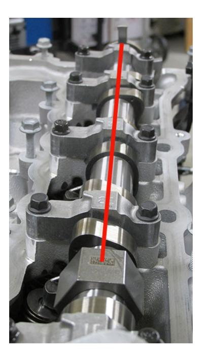
If you find the vacuum pump drive lugs are broke and/or the exhaust camshaft reluctor is out of position then replacement of the exhaust camshaft and vacuum pump will be required.
