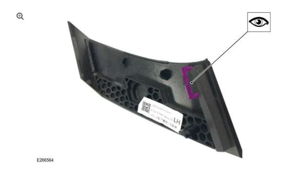
Inspect the retaining clip on the left windshield molding bolt cover.
