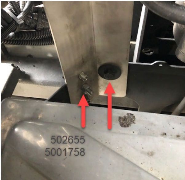
FIGURE 30: INSTALL FILTER DRYER POST
