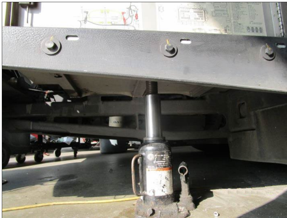
FIGURE 12: SUPPORTED BATTERY TRAY
