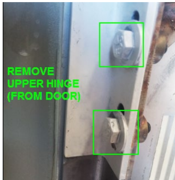
FIGURE 4 UPPER HINGE REMOVAL DOOR SIDE
