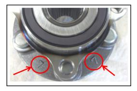
**NOTE:** The new part can be easily identified by "7"s made onto the back of the flange as shown here.
