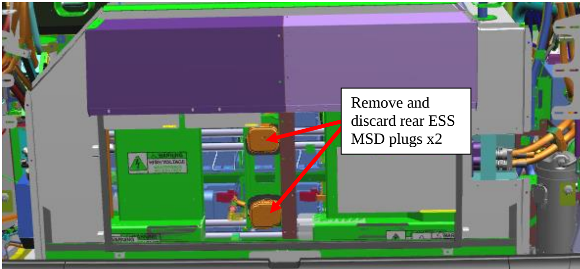
Figure 7: Rear ESS MSDs
