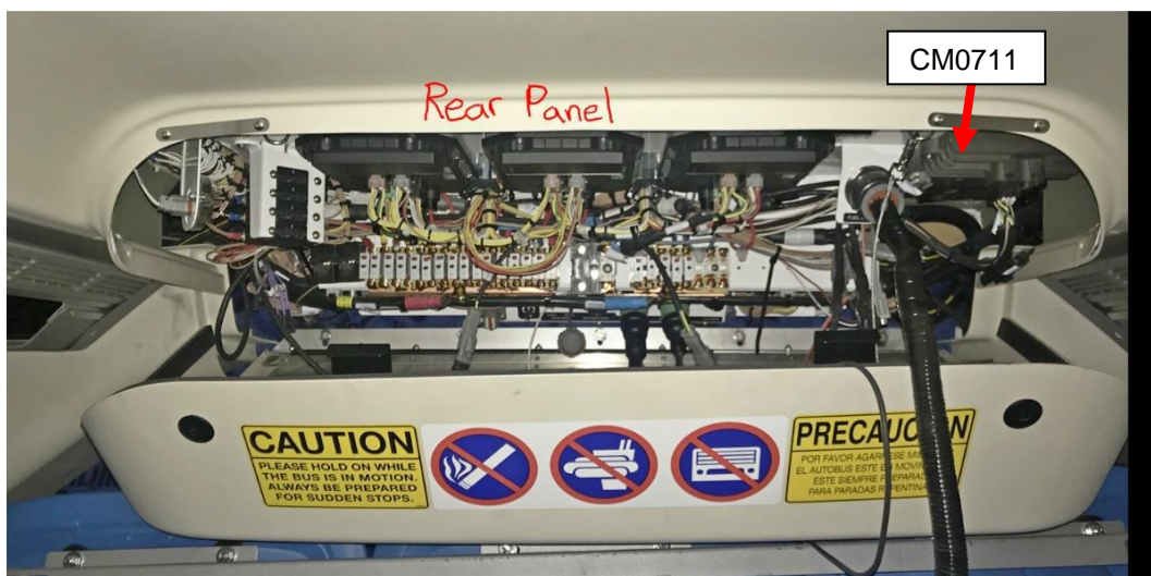
Figure 5: Rear panel and CM0711 module location
